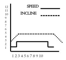
The **Warm Up Program** is designed to gradually increase the treadmill Speed and Elevation in the first segment (warm up) and gradually decrease the treadmill Speed and Elevation in the last segment (cool down). This is also known as a Plateau program.
